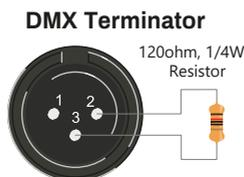
The DMX terminator is simply an XLR connector with a 120Ω (ohm), 1/4 Watt resistor connected across Signal (-) and Signal (+), respectively, pins 2 and 3, which is then plugged into the output socket on last projector in the chain. The connections are illustrated below.
