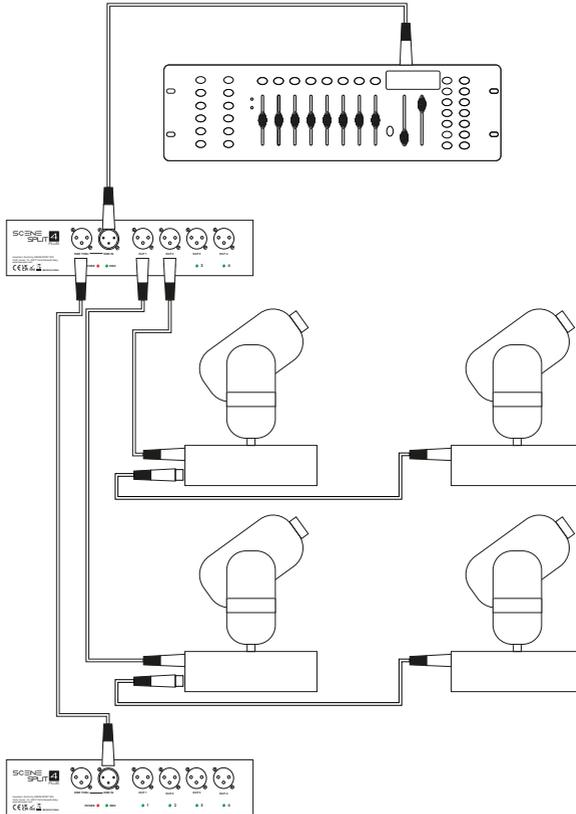
Connect fixtures using shielded 2-conductor twisted pair cable with 3-pin XLR male to female connectors. The shield connection is pin 1, while pin 2 is Data Negative (S-), and pin 3 is Data positive (S+).
