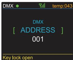
When the temperature indicator on the top-right corner changes from white to yellow, it means that the temperature has exceeded the maximum default settings.
