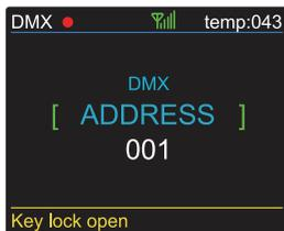
When the DMX icon is red, but Wireless icon is green, it means that DMX Mode is disconnected, but Wireless is connected.
