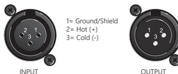
In case of unbalanced use, pins 1 and 3 will be bridged
