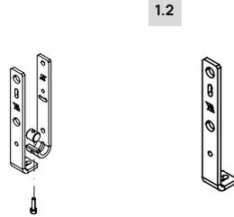
The bracket's plate with the flatter end is the one that gets mounted on the wall, acting as the base for the other bracket. Thanks to a freely rotating washer, the second bracket allows the speaker to be easily tilted to the desired angle.
