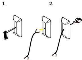
3. Connect the wires to pins 1 - 4 of the provided Euroblock connector and plug it to the speaker's terminals.
