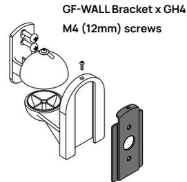
3. Mount the bracket to the rear panel of the speaker using the dedicated M4 screws provided
