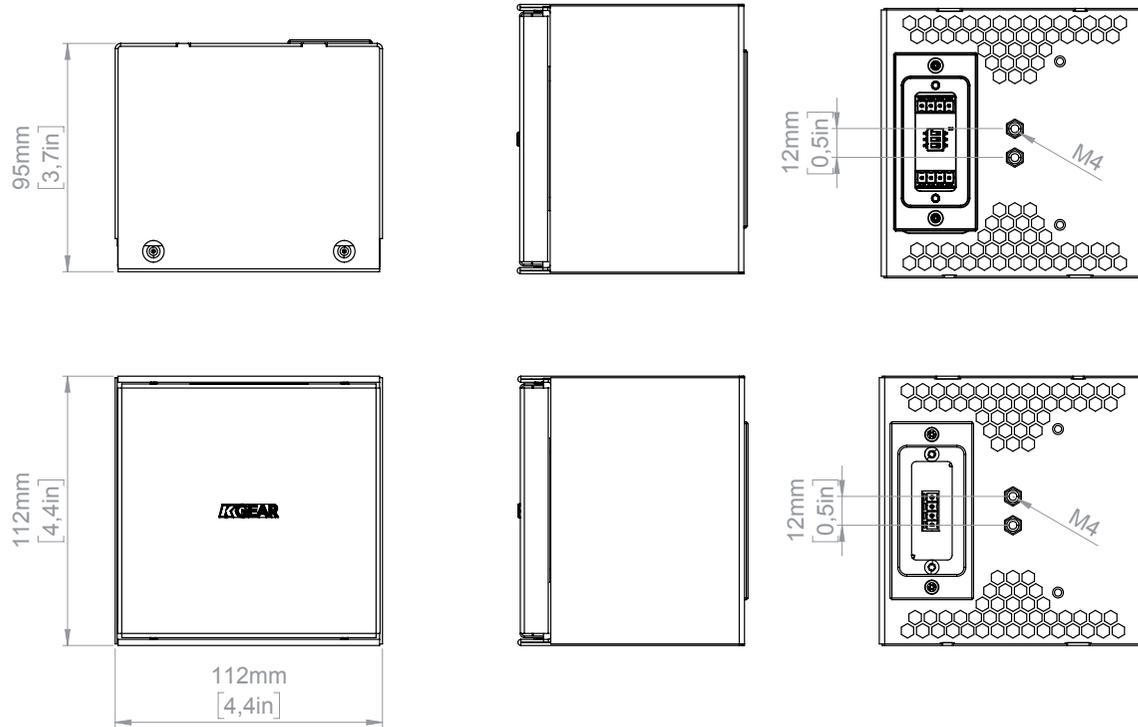
Mechanical Drawings - GF-WALL
