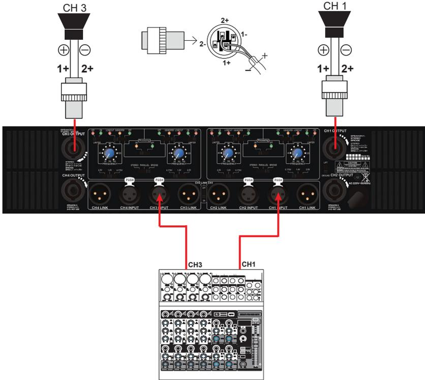
BRIDGE MODE with a mono input and a mono output, allows you to add the respective signals of the two amplification channels and make them available on a single output. The input signals of channel 1 and channel 3 will be sent respectively to CHANNEL 1 OUTPUT and CHANNEL 3 OUTPUT. Use the channel 1 and channel 3 controls to adjust the volume.
