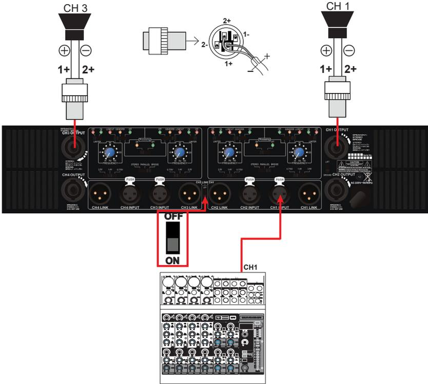
If the switch CH3 LINK CH1 is in ON position you can configure the amplifier with 1 input and 2 outputs. In this case CH1 must be the input. Please connect the outputs as shown above.
