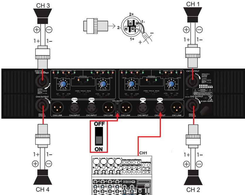
If the switch CH3 LINK CH1 is in ON position you can configure the amplifier with 1 input and 4 outputs. In this case CH1 must be the input. Please connect the outputs as shown above.
