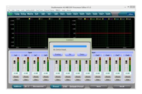
2, Connect the processor to the computer by USB, after turning on the device, the computer will searching new hardware automatically, during setup new hardware there will show the. Warnings: hardware setup success and can be used.
