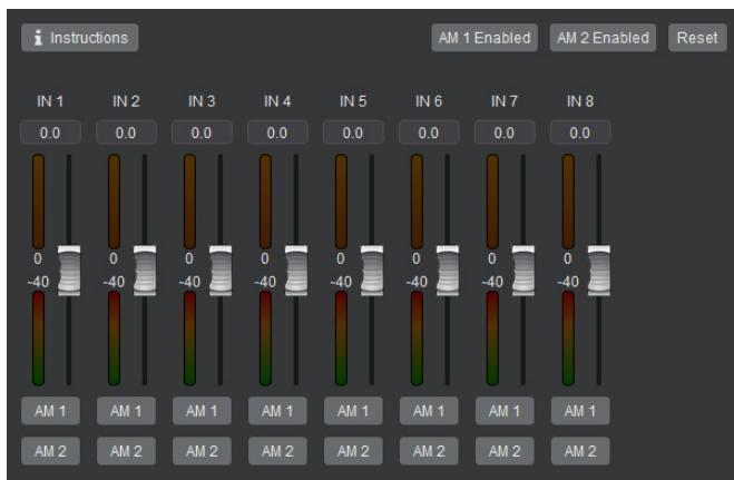
Automatic mixing algorithm is usually used in multi-microphone conference systems, which can effectively avoid Larsen effect when multiple microphones are turned on at the same time.
