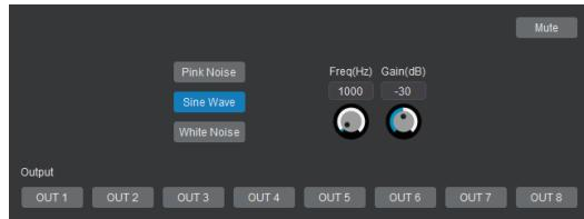
The signal generator supports pink noise, sine wave and white noise, which can be distributed to any output.
