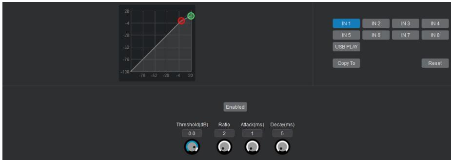
This processor supports an independent input limiter for each channel, and the activation, threshold, ratio, attack time and decay time can be adjusted. The limiter parameter can be copied and pasted quickly, which greatly improves the operation efficiency.
