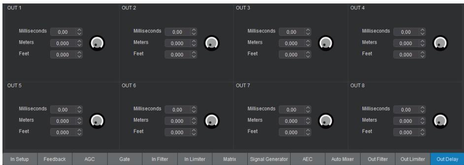
Each output channel has an independent delay, and the maximum delay time can be set to 300 milliseconds.
