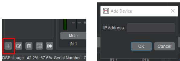
Try adding the device manually. Click the “+” icon in the lower-left corner, or right-click within the device list and select “Add Device.” A window will pop up—enter the device’s IP address to complete the addition. For example, the device’s IP address is 192.168.1.128
