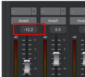
You can also click and type the keyboard up/right, down/left direction keys to achieve 0.1 dB step and step reduction. For complex parameter adjustment such as PEQ and Limiter, parameters can be copied and pasted quickly, and you can easily realize multi-channel data replication with convenient operation.
