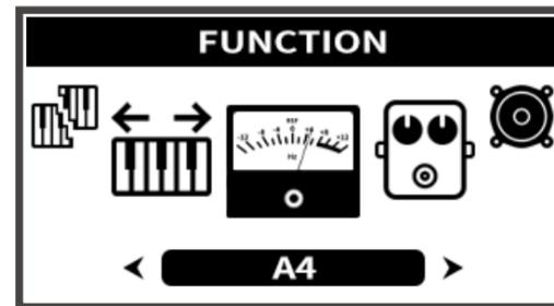
Turn the **[VALUE]** knob to adjust the A4 (425Hz-455Hz) and press the knob to confirm.
