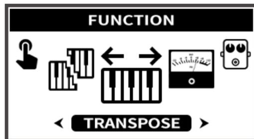
Turn the **[VALUE]** knob to Transpose in semitone steps ( $\pm 12$ ) and press the knob to confirm.
