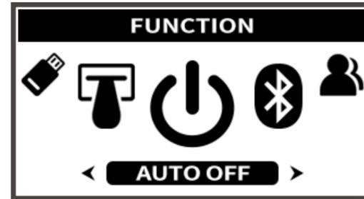
Use the [VALUE] knob to change the Auto Off settings. The NCK-330 will automatically power off if no buttons/keys are operated for a certain time (30min, 1hr, 2hrs, 3hrs, 4hrs).
