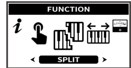
Turn the **[VALUE]** knob to select Left Keyboard or Right Keyboard, and press to enter the settings to adjust its Volume and Octave.
