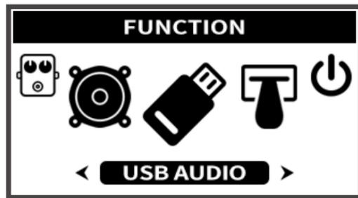
Turn the [VALUE] knob to adjust USB AUDIO Recording Level and press the knob to confirm.
