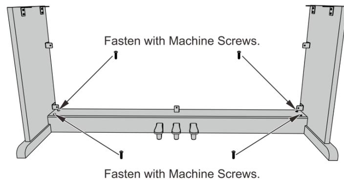
2. Attach the Rear Board to the Side Boards.
