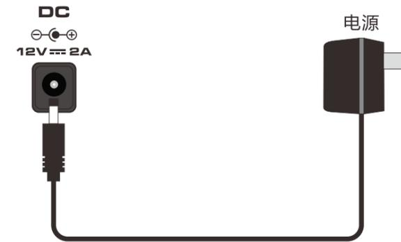
Connect the included power adaptor to the DC 12V jack and plug it to a power supply, the NCK-330 will be ready to be powered on.
