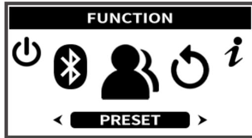
Use the [VALUE] knob to select a User Preset slot (5 User Presets in total). Press the knob to Save the preset to the current slot, or Load the saved preset.
