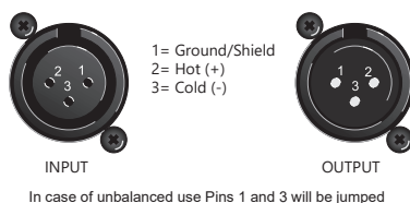
Balanced use of XLR connectors
