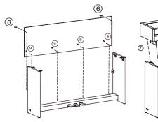
B. Place the back board against the stand completed in Step A, then use screw (9) and screw (6) to fix it to the stand.
