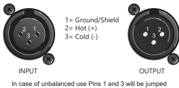
Balanced use of XLR connectors
