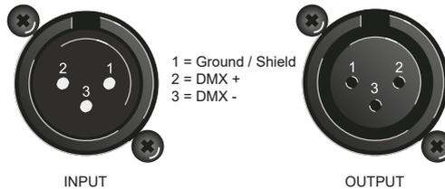
If you are using the recommended controllers, you can connect the DMX-output of the controller directly with the DMX-input of the first fixture in the DMX-chain. If you wish to connect DMX-controllers with other XLR-output, you need to use adapter-cables.
