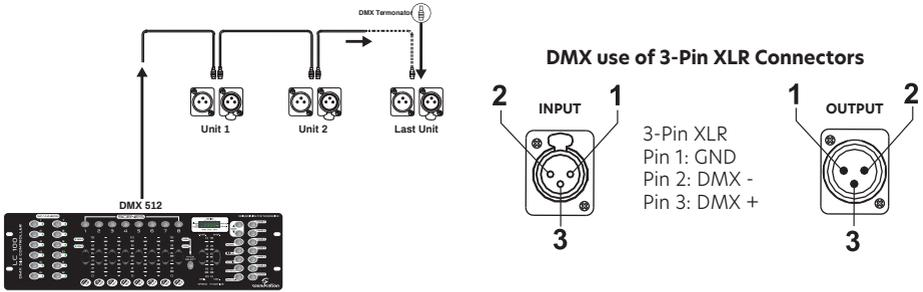
Connect machines using shielded 2-conductor twisted pair cable with 3-pin XLR male to female connectors. The shield connection is pin 1, while pin 2 is Data Negative (S-), and pin 3 is Data positive (S+).
