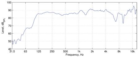
Frequency response (Anechoic measurement)
