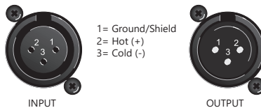
Balanced use of XLR connectors
