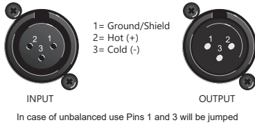
Balanced use of XLR connectors
