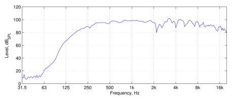
Frequency response (Anechoic measurements)
