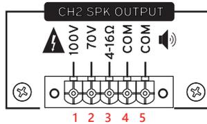
Each channel has a 5-pole Phoenix (Europlug) connector for connecting to loudspeakers.
