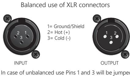
You can, of course, also connect unbalanced equipment to balanced inputs. Use either mono and stereo jack, making sure ring and collar are connected together (or pins 1 & 3 in the case of XLR connectors).
