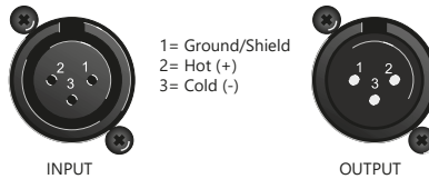
Balanced use of XLR connectors
