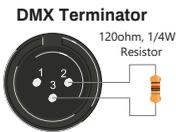
DMX is a resilient communication protocol, however errors still occasionally occur. In order to prevent electrical noise from disturbing and corrupting the DMX control signals, a good habit is to connect DMX output of last fixture in the chain to a DMX terminator, especially over long signal cable runs.
