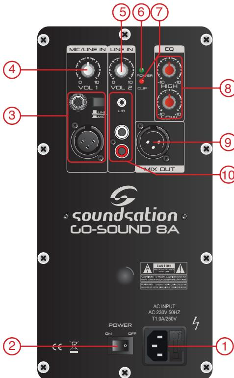
Plug the line-cord into an AC socket properly configured for your particular model. In case of fuse burn, to prevent the risk of fire and damaging the unit, please use only of the recommended fuse type as described in the manual. Before replacing the fuse, make sure the unit turned off and disconnected from the AC outlet.
