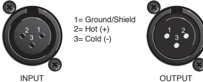
In case of unbalanced use Pins 1 and 3 will be jumped
