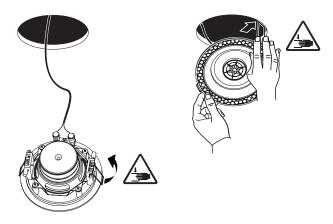
6 Lift the other clamp and insert in into the hole in order to set the loudspeaker in its final position.
