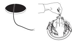
Lift one clamp of the loudspeaker and insert it into the hole paying attention to not hurting the hands.
