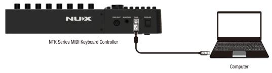
2. Press and hold the **DAW Button** to enter the DAW Mode, and use the encoder to select **CUBASE**.
