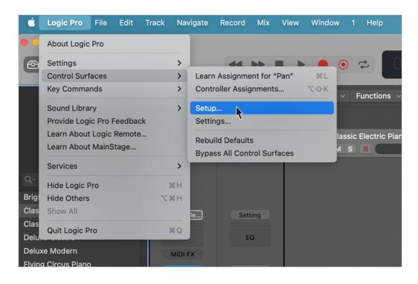
b. In the [Control Surface Setup] window, click [New], then select [Mackie Designs - Mackie Control] in the pop-up [Install] window and click [Add]. Go back to the [Control Surface Setup] window, select NUX NTK-XX Mackie/Hui for both the [Input Port] and the [Output Port].
