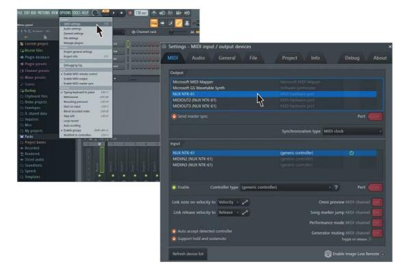
b. Next, select MIDIOUT2 (NUX NTK-XX) for [Output], then set the [Port] value to 0 and turn on [Send master sync]. Select MIDIIN2 (NUX NTK-XX) for [Input], then set [Controller type] as [Mackie Control Universal], set the [Port] value to 0, and turn on [Enable].
