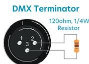
The DMX terminator is simply an XLR connector with a 120Ω (ohm), 1/4 Watt resistor connected across Signal (-) and Signal (+), respectively, pins 2 and 3, which is then plugged into the output socket on last projector in the chain. The connections are illustrated below.
