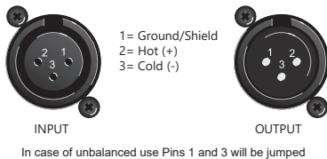
Balanced use of XLR connectors
