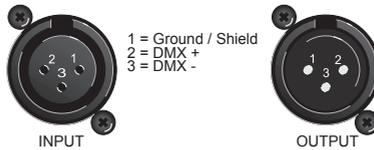
If you are using the recommended controllers, you can connect the DMX-output of the controller directly with the DMX-input of the first fixture in the DMX-chain. If you wish to connect DMX-controllers with other XLR-output, you need to use adapter-cables.
