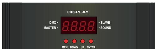
There is a 4-digit LED display, which shows names and value of all parameters during set up, and 4 buttons: MENU, DOWN, UP, ENTER.
